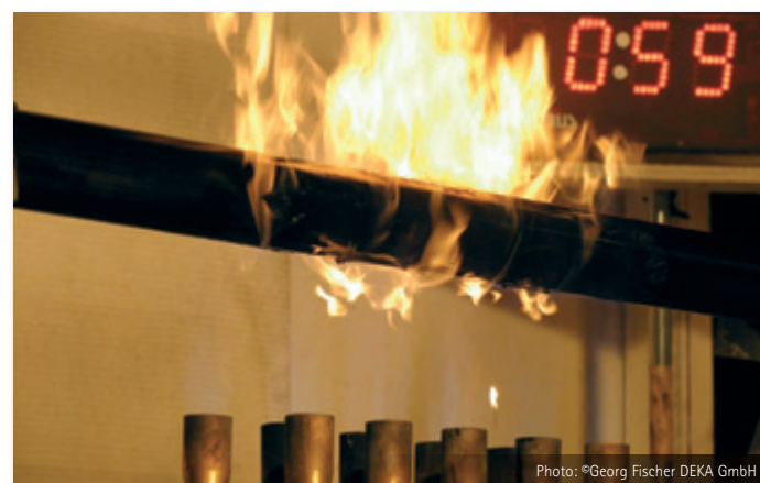
Fire test on a plastic pipe in accordance with the IMO 753 standard
