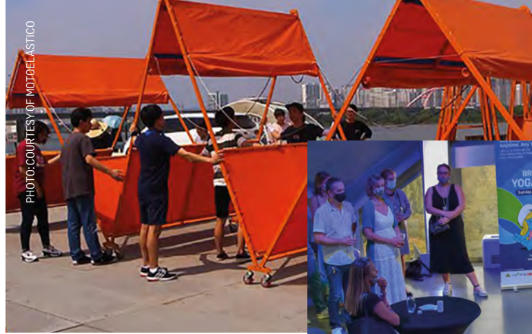
An example of flexible and functional structure, easily collapsible, stackable, and re-usable for temporary markets, made with PVC tarp.
